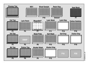
Figure 1. Example deck layout of the Biomek® FX instrument. Layout for the MagneSil® Blood Genomic, Max Yield System. Deck layouts may be different on different instruments and depend upon the individual instrument's configuration.
